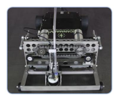
Using a single 10mm diameter short pulse 5MHz transducer mounted in a water column the ScanmapVS is effectively a remote access immersion system. Sampling every 6mm in the direction of travel ensures that all corrosion is mapped while maintaining continuous forward motion.
