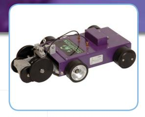
The Scorpion B-scan is a rugged remote access ultrasonic crawler designed to allow cost effective A and B-scan imaging on above ground ferro-magnetic structures without the need for costly scaffolding or rope access.
