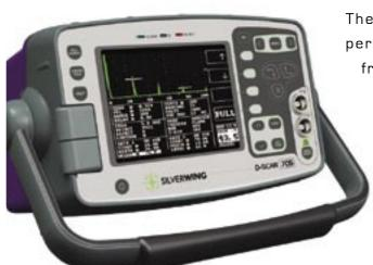
The D-SCAN 701 and 705 units are high performance digital ultrasonic flaw detectors from Silverwing UK. The latest developments in amplifier and pulser technology deliver higher levels of near surface resolution penetrating power and excellent signal to noise ratio. Typical applications are weld inspection, corrosion testing, small castings/ forgings and lamination checking.
